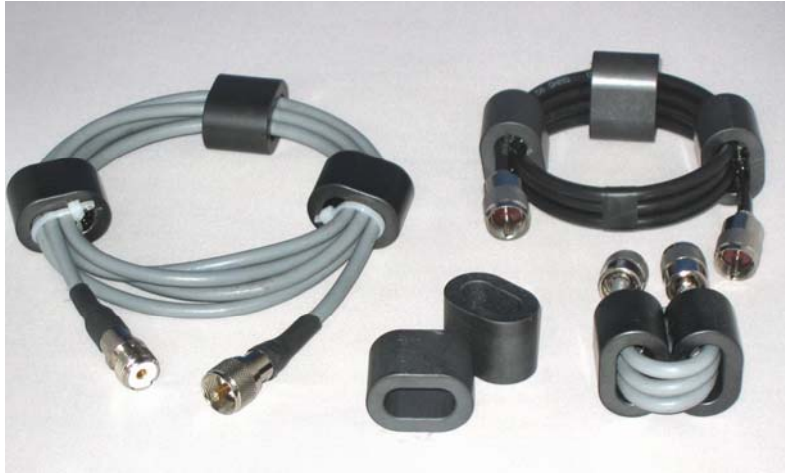
PHOTO 1: Clockwise from left: low-bands ferrite choke, mid-bands choke, high-bands choke and the ferrite cores.
